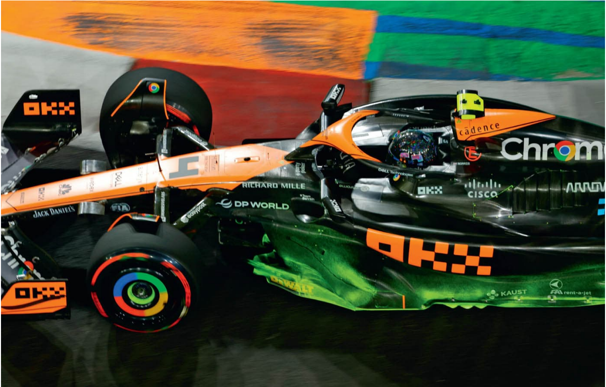
Stage three of the MCL60's conceptual upgrade, a total reprofiling of the sidepods with a steeply dished internal curve, was held back until the Singapore Grand Prix.
