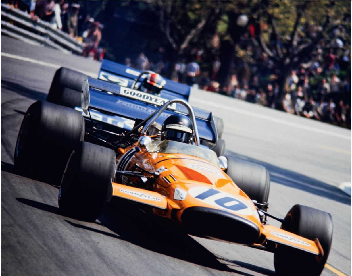
Goodyear had introduced an almost treadless tire at the 1971 season opener, but Firestone hit back with a full “slick” in Spain a month later.
