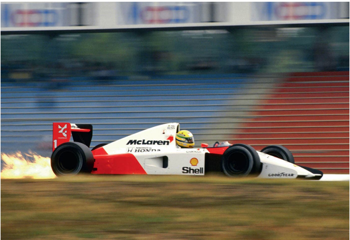
Ayrton Senna's MP4/6 spits flames at Hockenheim in 1991. Metering issues with Shell's new fuel blend proved costly midseason.
