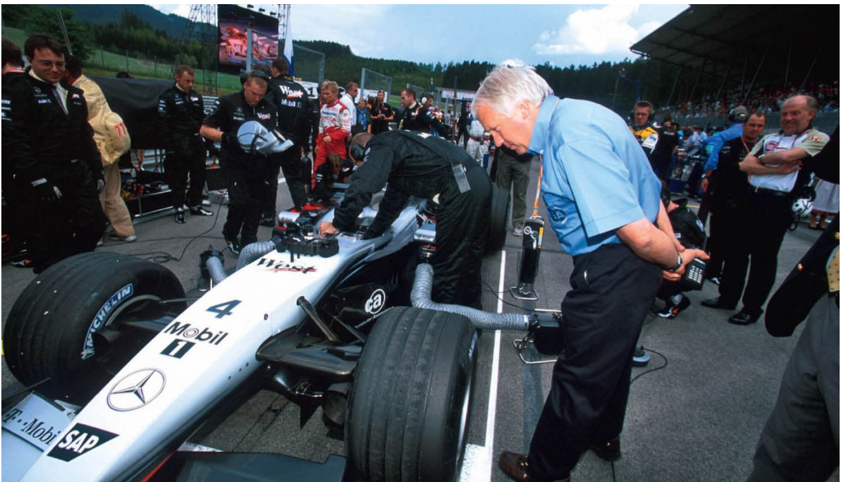
Charlie Whiting, the FIA's race director and technical delegate (jobs fulfilled by at least three people in the modern era) examines the MP4-17's front suspension on the grid in Austria. The complicated lower-wishbone arrangement offered aerodynamic benefits but compromised rigidity and suspension geometry.
