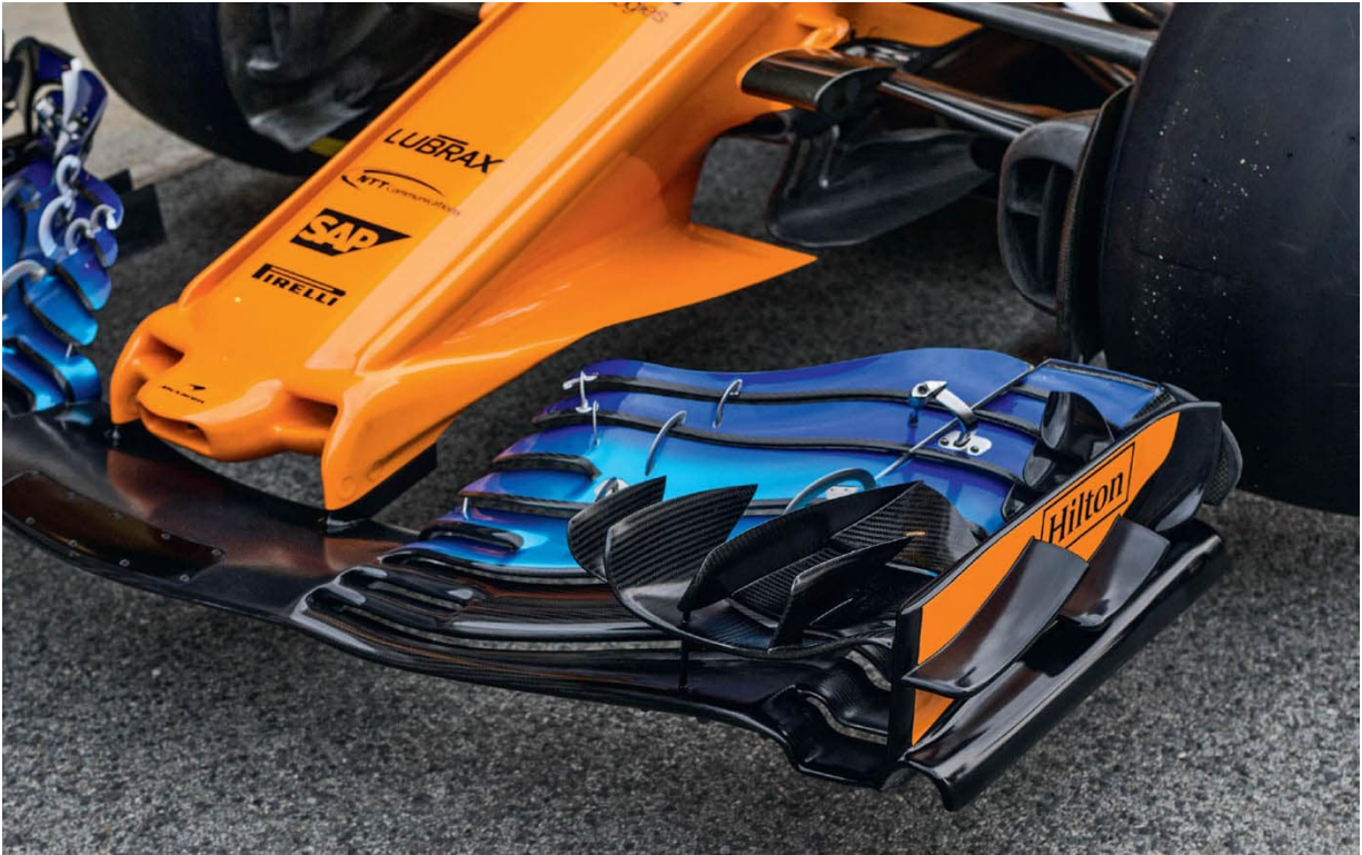
A more elaborate nose and front wing with lateral channels and a pronounced “cape,” fitted at the start of the European season, failed to deliver on expectations.
