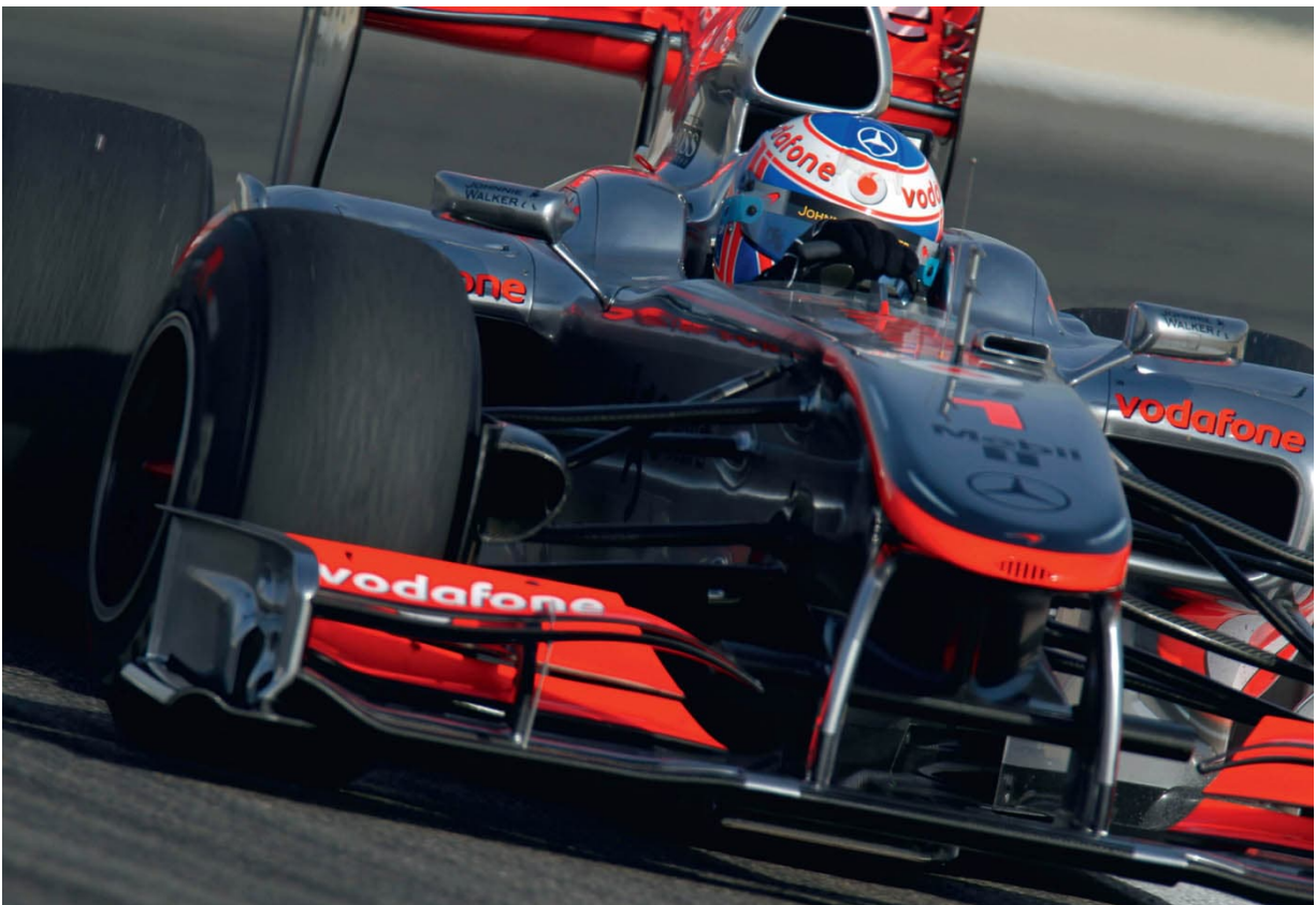
Jenson Button in the season-opening Bahrain Grand Prix. The air intake for the F-duct is visible to the immediate left of the mirror.
