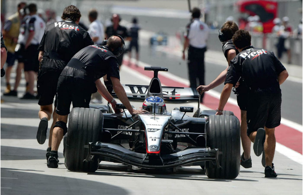
By round three, at the new Bahrain circuit, McLaren had dropped the multicurve front wing in favor of a simpler design.
