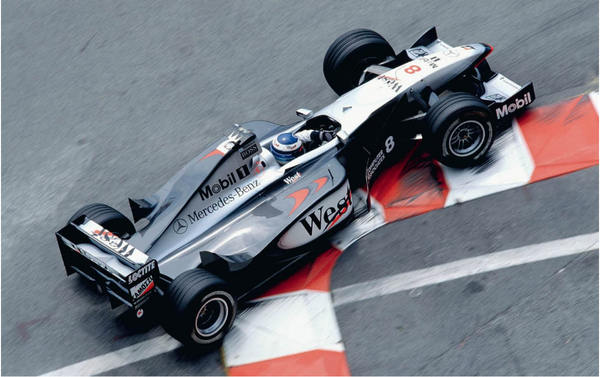
Elongated sidepods, combined with curving bargeboards, encouraged turbulent air behind the front wheels to wash away from the car.
